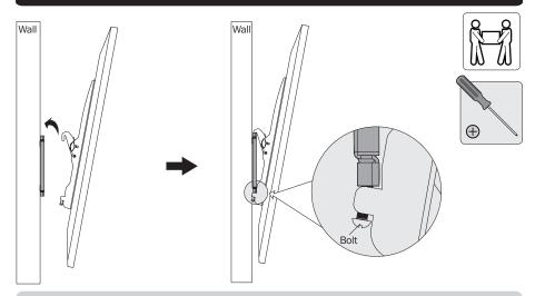
Tighten bottom bolts to secure display brackets to the wall plate.
